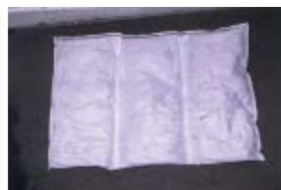
Commercial bag of oil sorbent (packed heated wood fibre).
