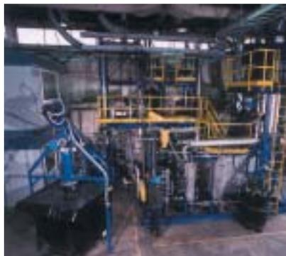
Figure 2: 10 t/d fluid bed fast pyrolysis plant in Vancouver.
