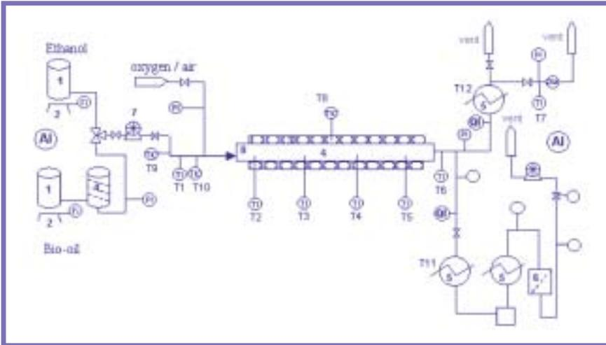
Figure 1: Entrained flow gasifier set-up.
