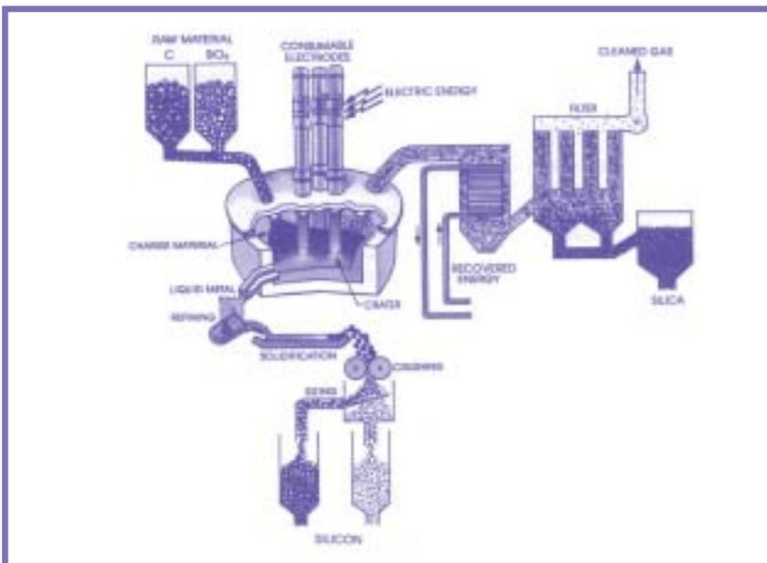
Figure 1. A typical plant for the production of silicon metal [1].
