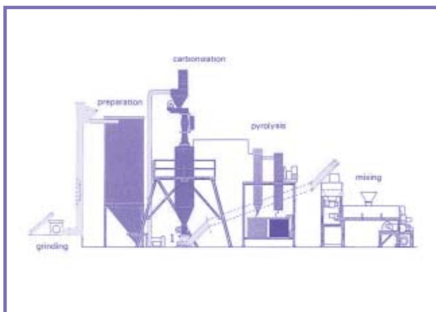
Figure 2: Process Schema for the Geneltec/BASA pyrolysis plant, as planned for NOVASEN.
