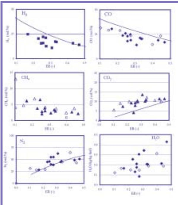
Figure 2: Dry gas composition upon bio-oil gasification using air at 1000°C (filled symbols) and 1100°C (open symbols). The solid lines represent theoretical values.
