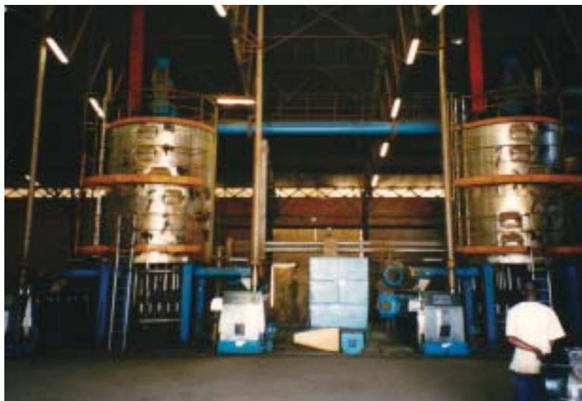
Figure 1: Detail of NOVASEN plant: Two conditioners (roasters) with screw presses where the oil is produced.
