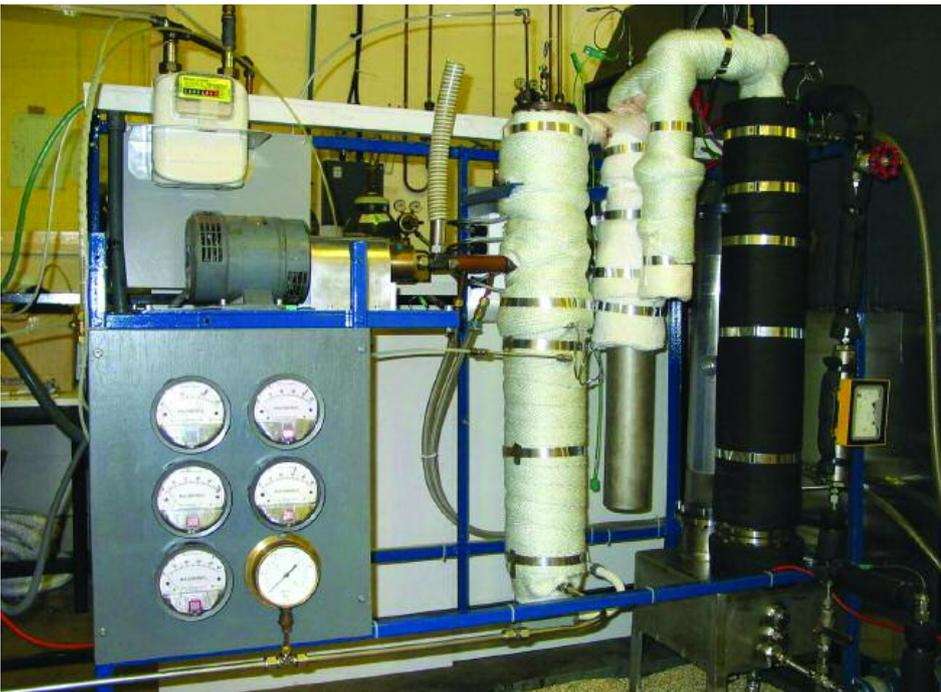
Figure 1: 1kg/hr fluidised bed pyrolysis rig with two cyclones, quench and electrostatic precipitator.
