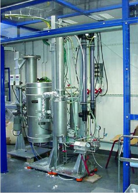
Figure 1: 1kg/h fluid bed pyrolysis unit.
