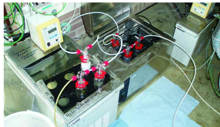
Figure 5: Sampling of reaction water and organic condensables according to the European Technical Specification for tar measurement in biomass gasification.
