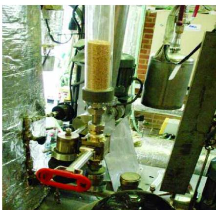
Figure 3: The feeding system for the pyrolysis rig at ECN.
