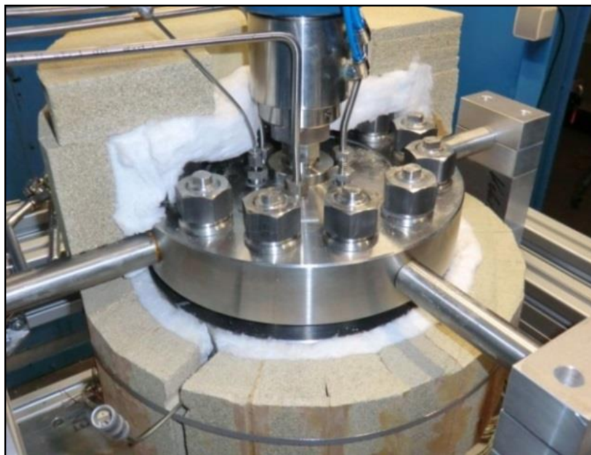
Figure 3: Stirred Tank Reactor 2000 ml, for temperatures up to 500 °C and pressures up to 300 bar
