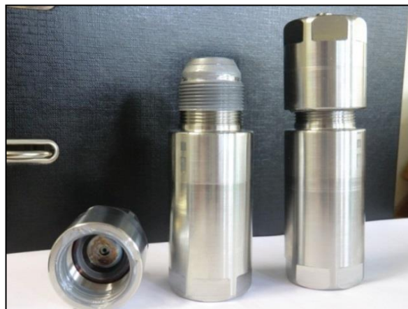
Figure 1: Micro Autoclaves 25 ml, stainless steel, for temperatures up to 500 °C and pressures up to 300 bar
