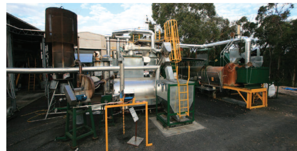
Figure 1: The 300kg/hour slow pyrolysis demonstration plant.
