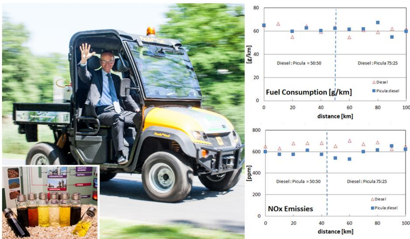
Figure 3: Top left: The JCB-Workmax UTV fuelled by a diesel–MTF mixture with Mr Kamp, Minister of Economic Affairs in the Netherlands. Right: Efficiency and emission levels during the 100 km trial (first 50 km 50:50; second 50 km 75:25). Bottom left: Products derived from pyrolysis liquids.
