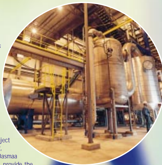
The vacuum pyrolysis reactor with the oil recovery system.
