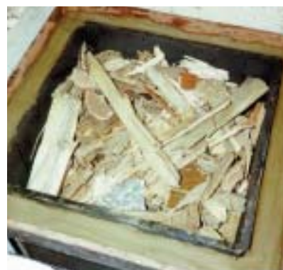
Figure 4: Contaminated wood in a thermolysis reactor.
