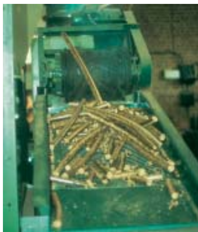
Figure 2: Briquettes production with a screw press.
