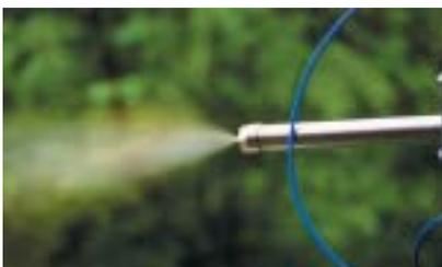
Figure 1: Typical spray cone with pyrolysis liquid (nozzle hole diameter 0.8mm; air pressure 2 bar and liquid flow 8 l/h).
