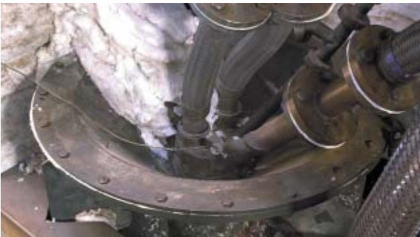
Figure 3: Hot sand and biomass feed to rotating cone pyrolyser.
