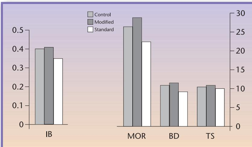
Figure 3: Tensile (IB) and bending (MOR) strength, 24h thickness swelling (TS) and bonding durability (BD) of pilot scale OSB produced with bio-oil modified PF resin.
