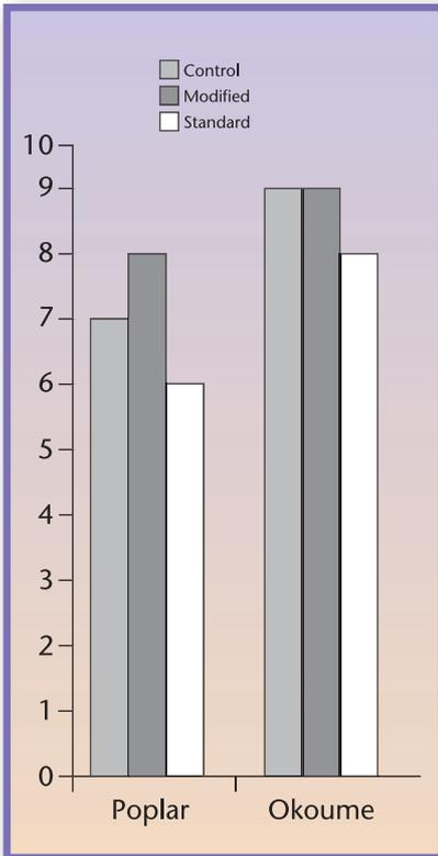
Figure 2: Bond quality of industrial plywood produced with bio-oil modified PF resin.
