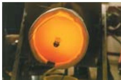
Figure 3: FLOX<sup>®</sup> burning chamber heated with pyrolysis liquid.
