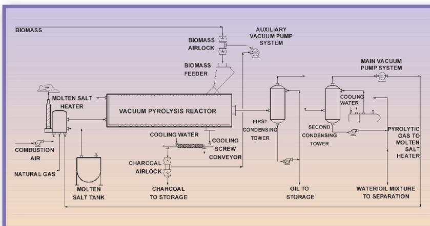
Figure 2: Pyrocycling™ process flow chart.
