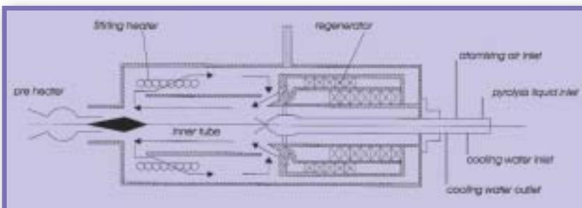
Figure 2: FLOX<sup>®</sup> burner pre heater and atomisation system assembly.
