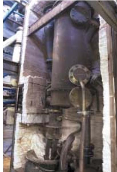
Figure 2: Char combustor with hot sand recycle to rotating cone pyrolyser.
