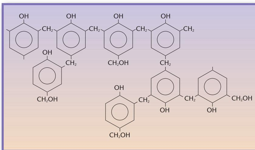
Figure 1: Resole structure.
