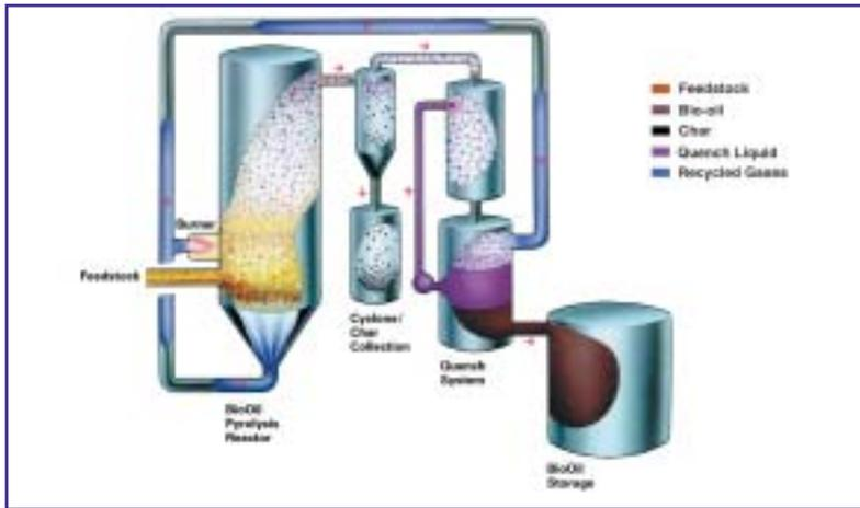
Figure 1: BioTherm™ flow sheet illustrating DynaMotives bio-oil production process.
