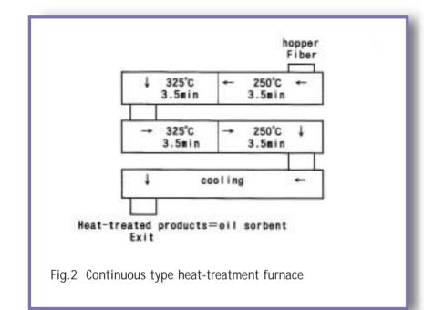
Figure 2: Continuous type heat-treatment furnace.
