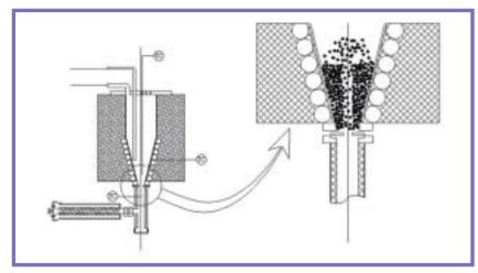
Figure 2: Spouted bed reactor.
