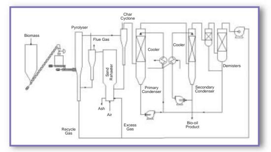
Figure 2: ENEL Fast Pyrolysis flowsheet.
