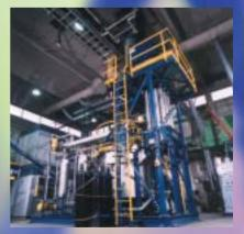
*Figure 1: 10 t/d fluid bed fast pyrolysis plant in Vancouver.*
