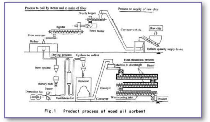
Figure 1: Product process of wood oil sorbent.
