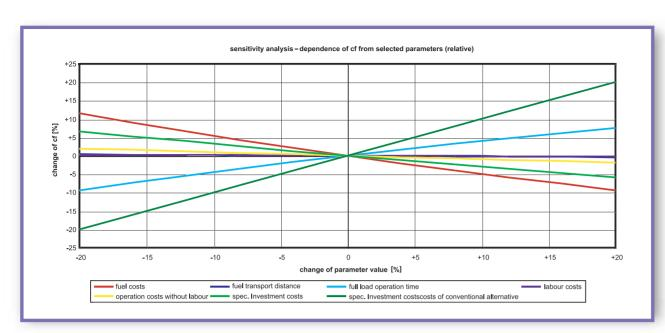
Figure 2: Sensitivity analysis – dependence of CF from selected parameters; Example Bio-oil Diesel CHP.
