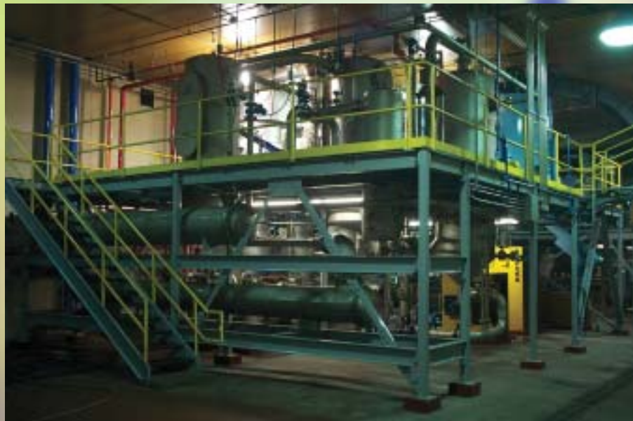
Figure 1: RTP™ 45 ton/day Wood Pyrolysis Plant.
