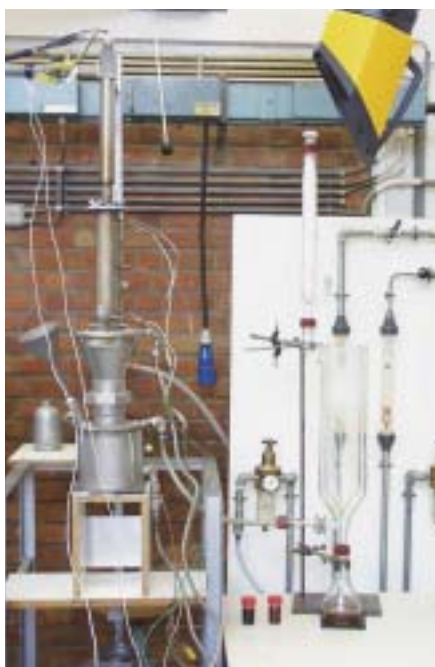
Figure 4: Experimental facility for the pyrolysis of wood chips: downdraft fixed bed reactor with gas cleaning system.
