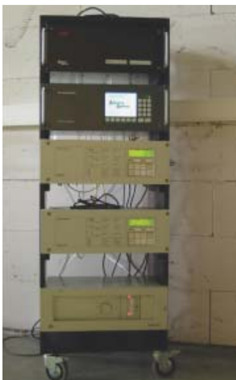
Figure 1: CRA – Pyrolysis gases analysing system.
