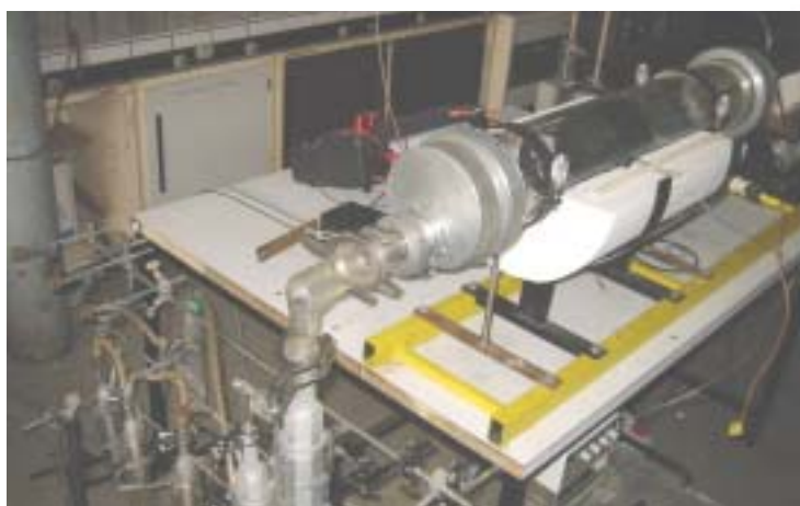
Figure 6: The laboratory batch rotating pyrolysis furnace (capacity 200g, up to 650°C).
