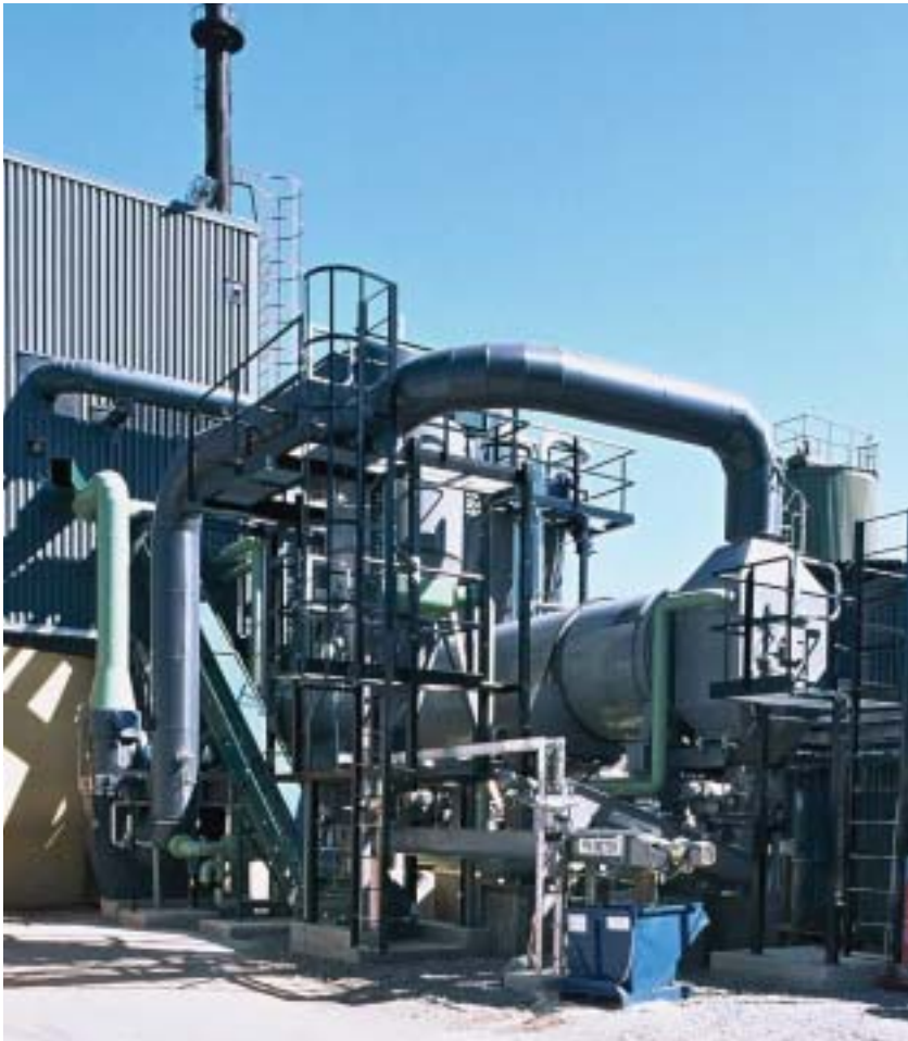
Figure 2: Forestera™ process flue gas drier.
