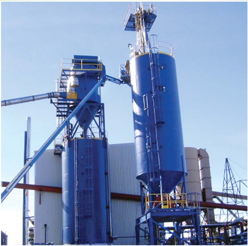
Figure 1: Wood feed hopper on left, char product hopper on right.
