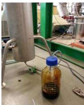
Figure 2: Intermediate pyrolysis of bamboo in a fully automated single screw auger reactor.
