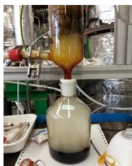
Figure 2: Intermediate pyrolysis of bamboo in a fully automated single screw auger reactor.
