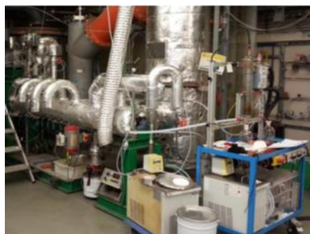
Figure 2: Intermediate pyrolysis of bamboo in a fully automated single screw auger reactor.
