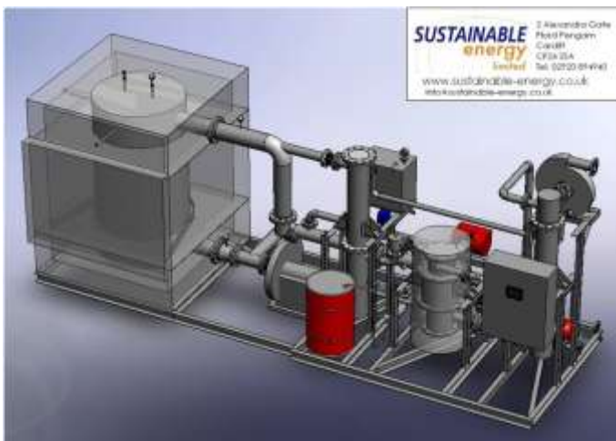
Figure 2: 3D CAD of IBERS slow pyrolysis reactor as designed by Sustainable Energy Ltd.
