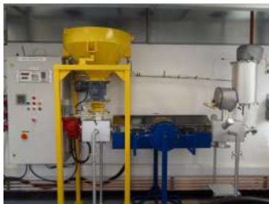
Figure 2: Continuous screw pyrolysis unit (5kg/h).
