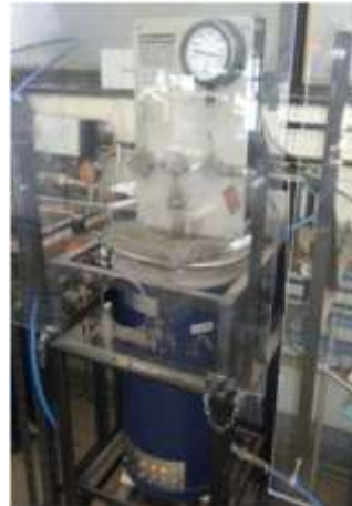
Figure 2: Apparatus for investigating hydrothermal treatment and solvent mediated thermolysis showing a pressure vessel immersed in a fluidized sandbath.
