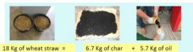
Figure 2: Output from larger scale microwave mediated pyrolysis of biomass.
