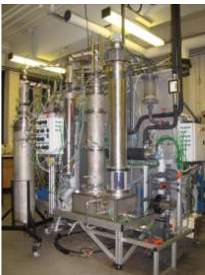
Figure 1: 7 kg/h continuous fast pyrolysis unit.
