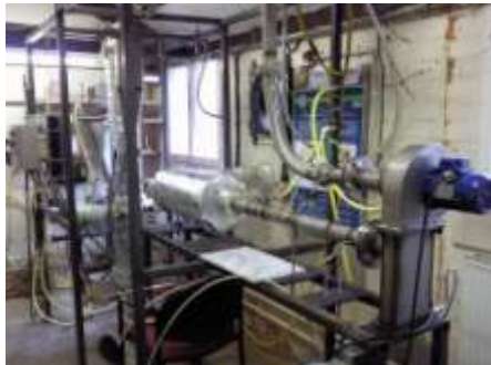
Figure 1: Laboratory-scale, electrically heated, bubbling fluidized bed biomass gasification system for processing.
