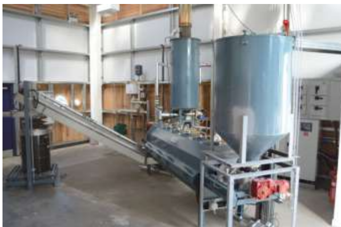
Figure 1: Pilot-scale pyrolysis unit (50kg/h).
