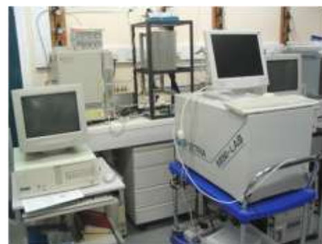
Figure 2: Plug flow reactor equipped with online GC/MS.
