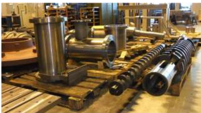
Figure 1: The new pyroformer technology for improved biochar and pyrolysis gas production – a 100 kg/h intermediate pyrolysis unit.
