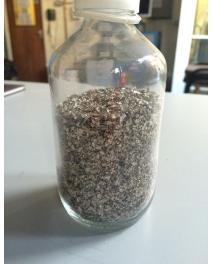
Figure 2: Aluminium recovered from laminated beverage packaging.
