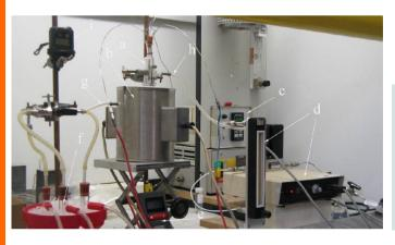
Figure 1: Bench scale experimental rig for catalytic pyrolysis.
