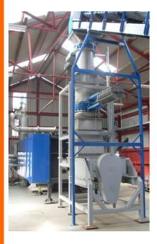
The system comprises automated material feeding, a core pyrolysis processor with a fully integrated gas management system challenges that exist which produces a gas clean enough for direct use in a reciprocating gas engine. This gives the EPi process the capability of elevated electrical efficiency when compared against
