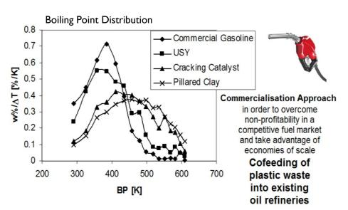
**Figure 2:** Boiling Point Distribution of liquid fuel from catalytic pyrolysis of polyethylene over various catalysts. Comparison with commercial gasoline (petrol).
