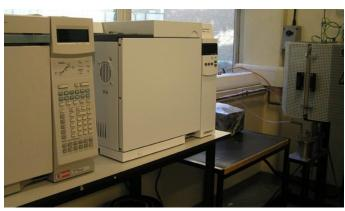
Figure 1: Pyrolysis equipped with online GCs.
