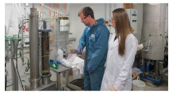
Figure 2: Aston's 1kg h<sup>-1</sup> continuous fast pyrolysis unit.
