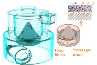
**Figure 1:** The TORBED<sup>®</sup> Compact Bed Reactor (CBR). Gas is introduced underneath the blades of the CBR leading to high velocity gas jets that fluidise and fully mix the bed maximising gassolid contact.
