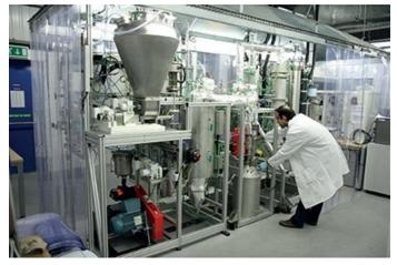
Figure 2: 5 kg/h fluid bed pyrolysis rig for Future Blends, UK.
