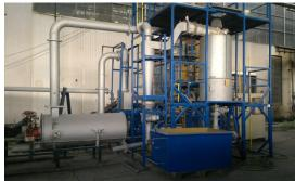
**Figure 2:** The 500 kWth TORBED<sup>®</sup> pilot test facility used to conduct thermal trials on a variety of sustainably sourced biomass and waste materials.
