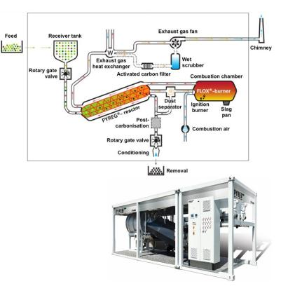
Figure 1: PYREG<sup>®</sup>P500 module and its schematic diagram.
