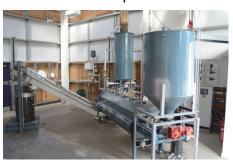
Figure 1: Pilot-scale pyrolysis unit (50kg/h).
