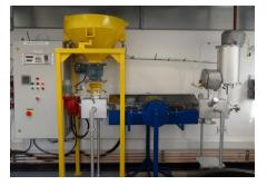
Figure 2: Continuous screw pyrolysis unit (5kg/h).
