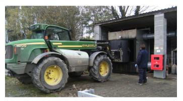
**Figure 2:** Loading of feedstock-filled stillage unit into unit for heating run.
