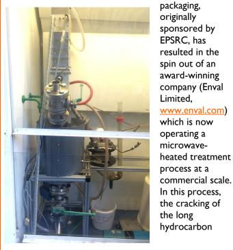
packaging, originally sponsored by EPSRC, has resulted in the spin out of an award-winning company (Enval Limited. www.enval.com which is now operating a microwaveheated treatment theres-aluminium-if-not-brass. The process has also been successful in processing other hydrocarbon-containing materials such as used automotive and marine oils, waste and virgin vegetable oils and polyethylene, to generate hydrocarbon fuels. In all cases, sufficient hydrocarbon gas can be
