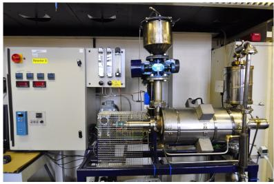
Figure 1: Screw kiln pyrolysis-gasification reactor.
