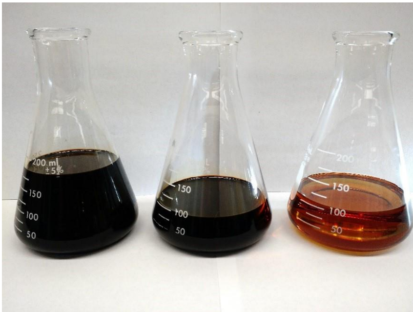
Fig. 3 - Acetone-free bio-oil from the solvent liquefaction process (left) is fed into the bio-oil fractionation system which separates the feed into a bottoms (center) and overheads (right) product, otherwise referred to as heavy bio-oil and medium oil, respectively.
