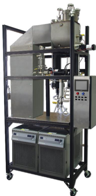
Figure 2: Mainstream's automated, continuous bench-scale pyrolysis unit.
