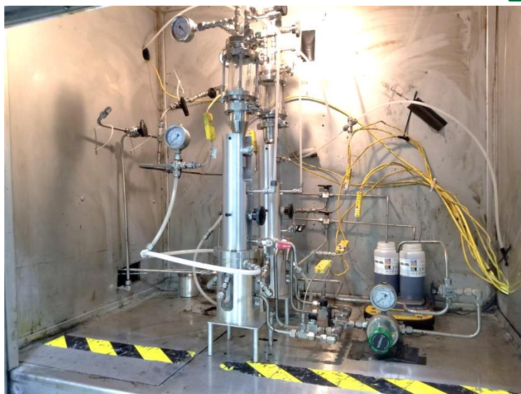
Figure 2: Bench scale cross-flow microfiltration system designed for solids/ash removal of FPBOs at CanmetENERGY
