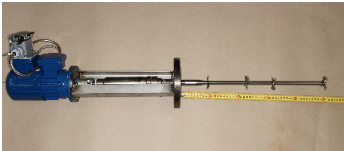
Figure 1: Mechanical mixer used in VTT's bench scale BFB reactor.
