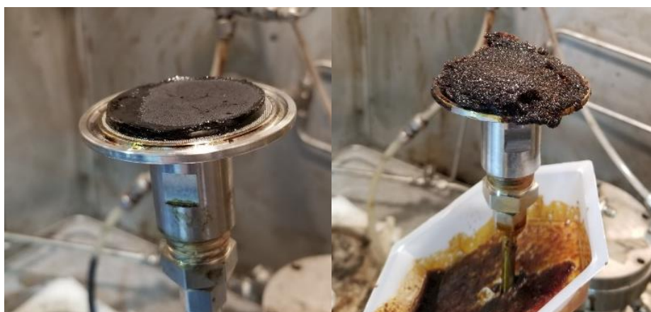
Figure 5: Filter "cake" leftover after dead-end microfiltration of FPBO (left) and FPBO + 5 wt% solid phase adsorbent (right) from testing combined solids/ash removal strategies
