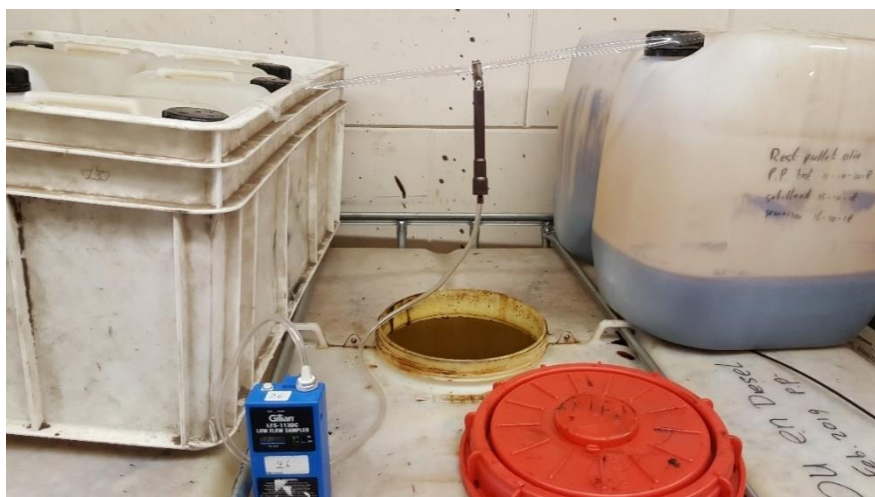
Fig. 15: photograph of formaldehyde measurement in the gas phase ‘worst-case scenario 3’
