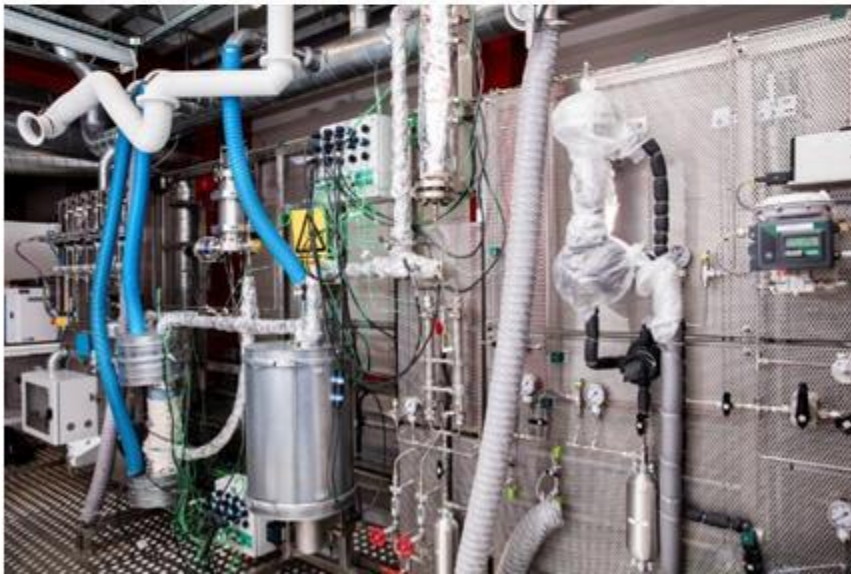
Fig: 3: Experimental setup at DTU-Chemical Engineering for catalytic hydrodeoxygenation of biomass with downstream hydrotreatment (HDO) for deep deoxygenation. Example of product directly obtained from the process is shown to the right with clean oxygen-free hydrocarbon phase on top and clean C-free water phase below. 4
