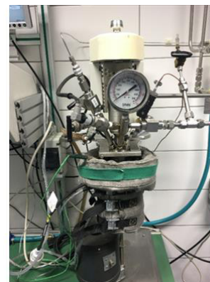
Fig. 2: Process flow chart of the lab-scale batch equipment (left) and 50-ml-reactor (Paar Instruments, series 4560) with heating wristbands, steering system and gas inlet and exhaust at the reactor head (right)
