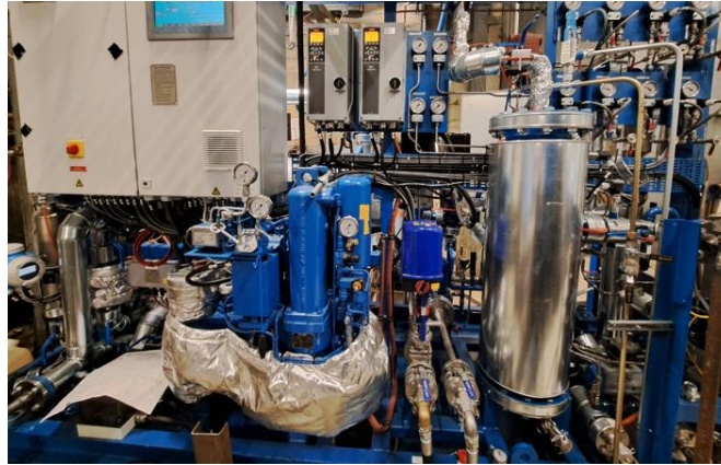
Fig. 1: The Auramarine feeder-booster fuel supply unit developed for test new drop-in replacement biofuels for testing.
