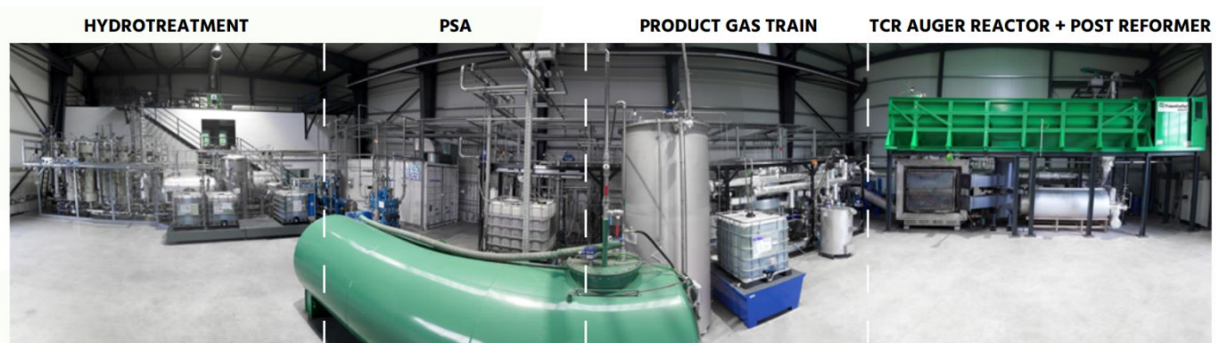
Fig. 2: Complete process chain of TO-SYN-FUEL-demonstrator. Credit: Fraunhofer UMSICHT
