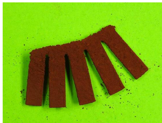
Fig. 13: Fins fallen off the economizer
