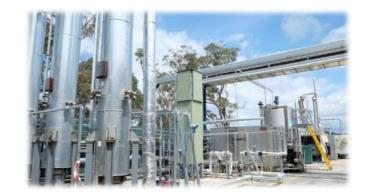
liquefaction technology trademarked as catalytic hydrothermal reactor (Cat-HTR<sup>TM</sup>). The company developed the technology to the demonstration scale (5,000 t/y) at Somerby in New South Wales, resulting in a potential production of 1.6 ML of renewable bio-oil. Subsequently Licella partnered with Canfor (Canada) to form the joint venture Arbios Biotech. The plant is used to refine and optimise the Cat-HTR™ process for a range of post-consumer biomass feedstocks.
