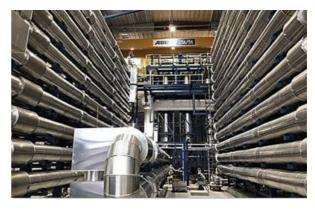
paper pulp, timber and bioenergy production. The construction of a EUR 50.6M demonstration plant was completed in November 2021 at the Statkraft Tofte site. The facility utilises Steeper Energy's hydrothermal liquefaction technology (Hydrofaction®) to convert forest residues into a bio-crude oil at a rate of 30 barrels per day (BPD). At commercial scale, Hydrofaction® design could incorporate independent parallel lines ranging from 200-800 BPD to achieve production levels in excess of 2,000 BPD.
