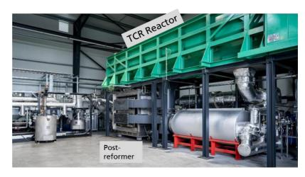
first stage, the biomass is converted by intermediate pyrolysis in an auger reactor. In a post-reformer, the solid residue and the vapours are catalytically refined at temperatures of up to 700 °C to improve gas yield and product quality. Condensed oil and process water are separated, and the permanent gas product is cleaned.
