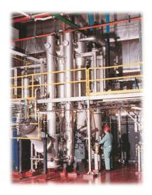
chemicals for the food industry and heating fuels. Liquid smoke, generated by the controlled pyrolysis of hardwood sawdust, is used to flavour and give anti-microbial benefits cross a range of applications, from beverages to desserts. The facilities utilise Ensyn's RTP® technology and receive ongoing operations supervision, maintenance and technical support from Ensyn.
