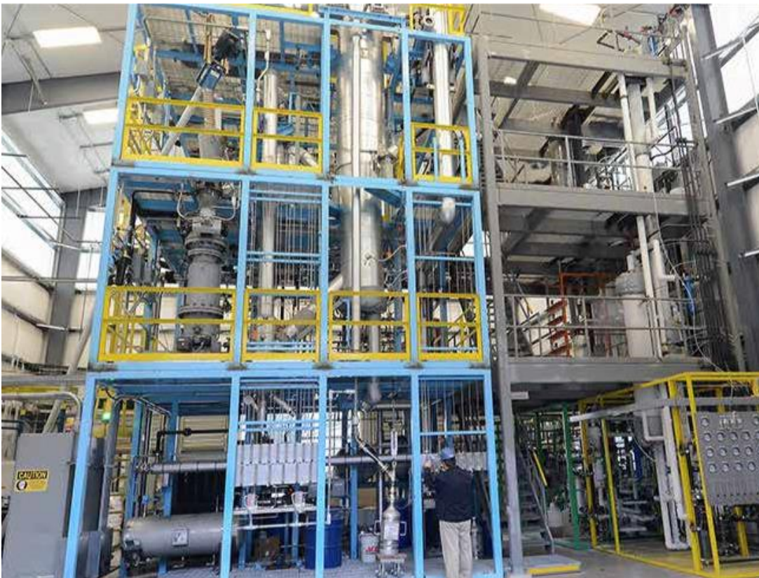
Fast pyrolysis pilot plant at RTI International in Research Triangle, North Carolina. The plant has a capacity of 1 tonne of dry biomass per day.
