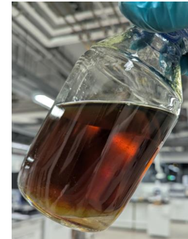
U-WCO after distillation
